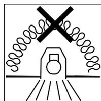
Luminaire not suitable for covering with thermally insulating material
