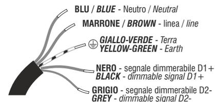
**64W/125W/252W** connettore/connector 7 x 1.5mm<sup>2</sup> IP65
