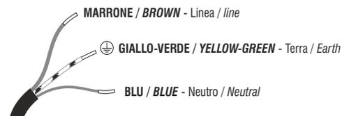
**125W/252W** connettore/connector 5 x 1.5mm<sup>2</sup> IP65
