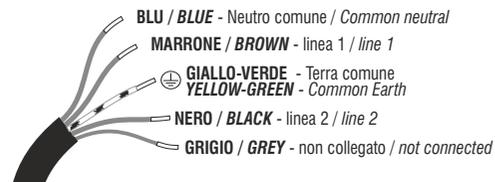
**64W/125W/252W** connettore/connector 5 x 1.5mm<sup>2</sup> IP65
