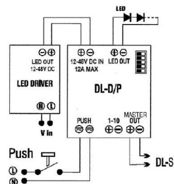
Schema/wiring Push 230Vac
