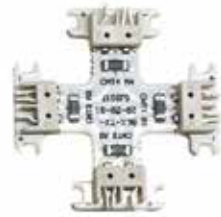
42AA07EL 4 ways electrified connector.
