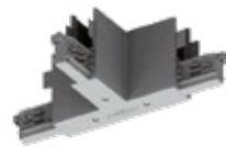
"T" coupler (internal 08 / external 06) 250V-50Hz max 16A - for H version.
