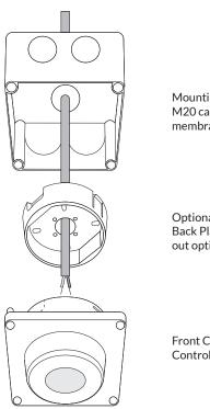
Mounting Box with M20 cable entry membrane options.
