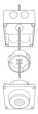
Mounting Box with M20 cable entry membrane options.
