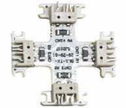
42AA07EL 4 ways electrified connector.
